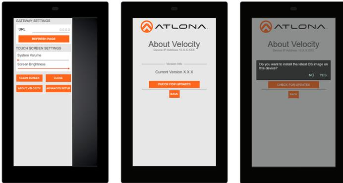
When the installation starts, it will switch to an Android update screen. Once completed it will restart the touch panel. The splash screen will appear, before the loading screen takes over. The update is complete when it returns to the control screen. This process can take up to 5 minutes to complete.
